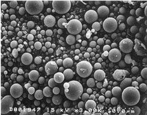
**FIGURE 3: ASH PARTICLE MAGNIFIED 2000X**
