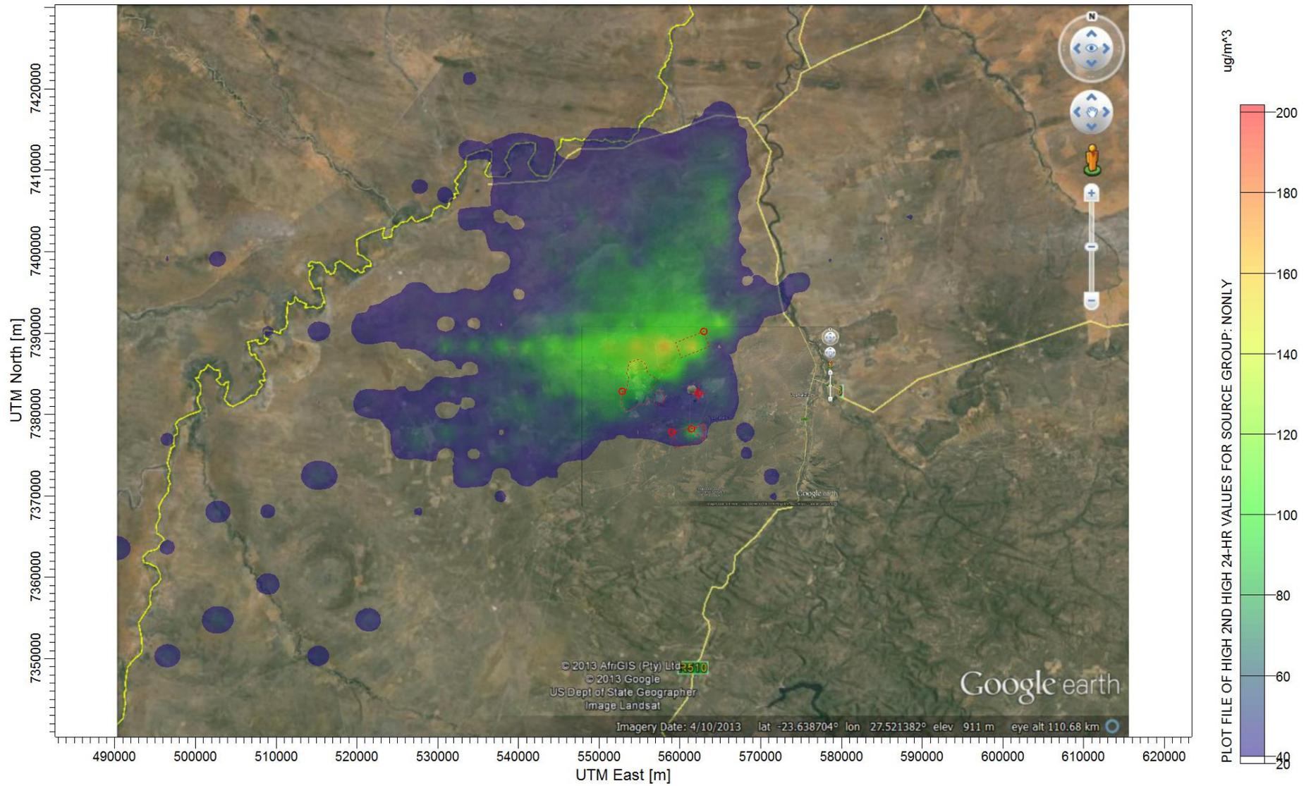
**FIGURE 19: DAILY AVERAGE PM10 CONCENTRATIONS AT SITE ALTERNATIVE 2 INCLUDING CONVEYORS**
